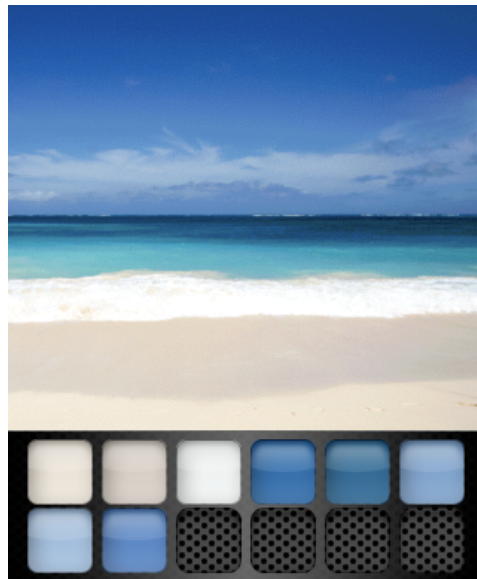
Figure 2. Color Palette organized by the order colors appear in an image (bottom-to-top). Images are sometimes processed bottom-to-top because of their memory layout.
